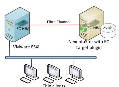
The following diagram shows a simple Target FC configuration.
