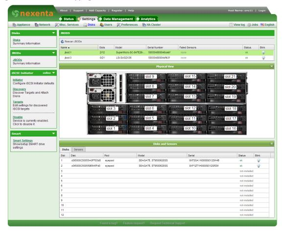
The slot map also displays the state of the disk and the occupied disk slots. The green light indicates that a disk is in a healthy state, the red light indicates that a disk is corrupted, or failed.
